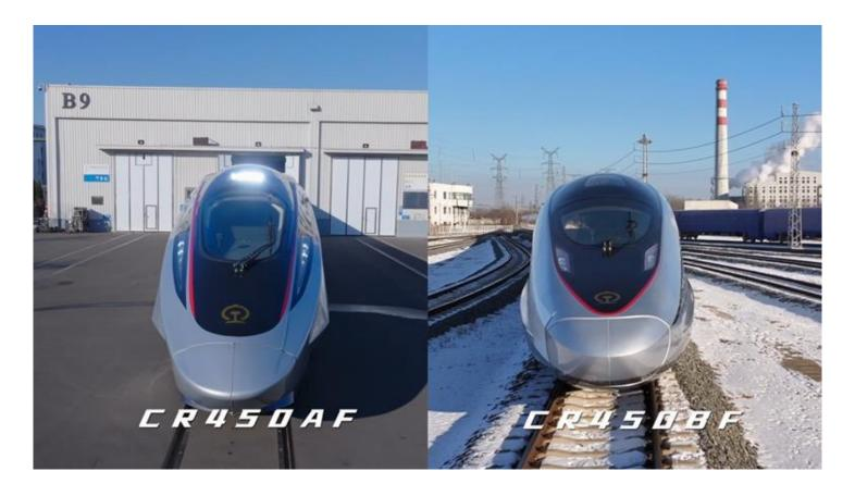
The CR450AF and CR450BF trainsets unveiled by CRRC and China Railway on December 29 each have four powered and four non-powered vehicles. They have a water-cooled permanent magnet traction system, and braking systems designed so the stopping distance is about the same as for trains running at a lower maximum speed. There are more than 4 000 sensors for the real-time monitoring of key systems.
