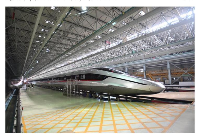
The CR450 is 10% lighter than the previous CR400. Measures to reduce drag include bogie enclosures to lower air resistance. The nose of one train is inspired by an arrowhead, and the other by an eagle in flight.
